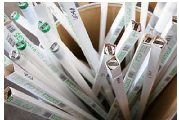
Fluorescent lamps contain mercury and must be recycled.
