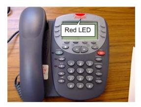
7) Once the phone has powered on, allow it to run through its bootup process. Eventually, it will log in to the PBX automatically. You will know it has successfully logged in when you see a 5 digit extension in the upper left corner and the correct date and time in the upper right corner.
