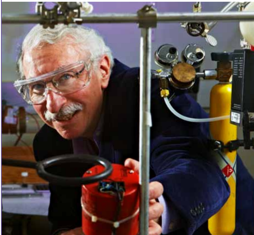
ABOVE: Buddy Ratner demonstrates the Radio Frequency Plasma System which modifies materials to create coatings for medical implants.
